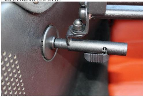
**STEP 5**Fold both rear seats forward and attach the supplied brackets to the rear of the seat using two self-tapping screws (not supplied). To determine exact position for click the wind deflector into the car and make sure the wind deflector is horizontal.
